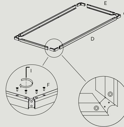
NB! Make sure the holes on the corner (C) are facing up.
