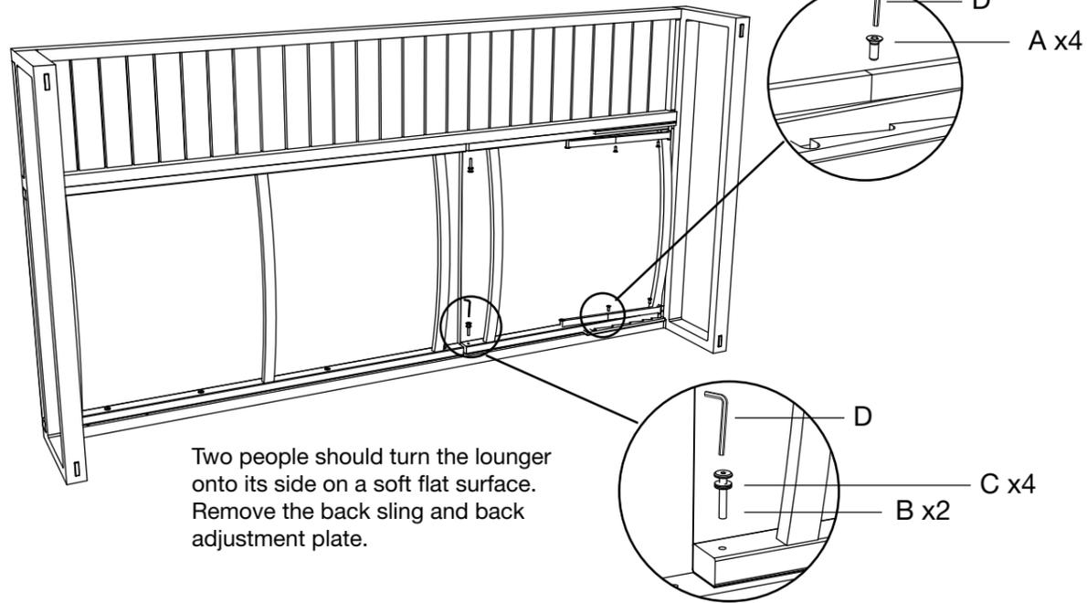
Two people should turn the lounge onto its side on a soft flat surface. Remove the back sling and back adjustment plate.
