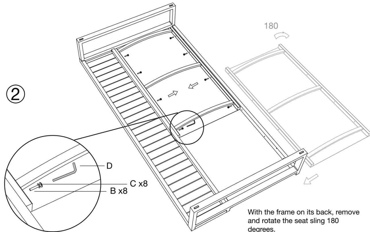
With the frame on its back, remove and rotate the seat sling 180 degrees.
