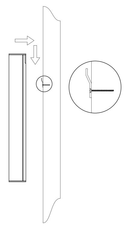
Step 3. Carefully take the mirror and lift ontop of the wall bracket so that the rear pannel of the mirror rests neatly up against the rubber pad of the bracket and make sure that it is roughly central on the bracket.
