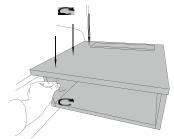
Turn all the three grub screws evenly out. You might need to pull the metal a little bit out of the DEPO.
