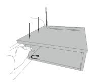
Turn all the three grub screws evenly out. You might need to pull the metal a little bit out of the DEPO.
