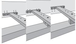
without distance block: insertion depth 14,5 cm horizontal distance block: insertion depth 12,5 cm standing distance block: insertion depth 10,5 cm Use the countersunk screws in the correct length (5x60/80)to fix the distance block.
