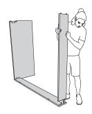
**2.** Attach the head and foot sections and fix them with grub screws.
