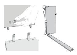
**1.** Screw the bolts into the long sides and insert the connector housing into the head and foot sections. Align bolts and housing correctly!
