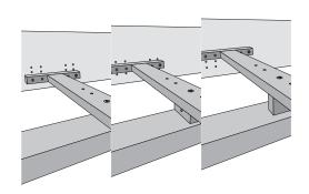
without spacer block: insertion depth 14,5 cm horizontal spacer block: insertion depth 12,5 cm standing spacer block: insertion depth 10,5 cm Use the countersunk screws in the correct length (5x60/80) to fix the spacer block.
