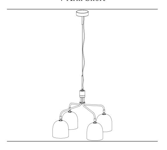
Connect lamp L and N wires to mains wires in the supplied screw terminal and place it inside the canopy.
