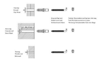
Template for drilling for mounting screws.
