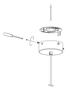
A: REMOVE SCREWS. B: PULL WIRE AND CUT IN DESIRED LENGHT.
