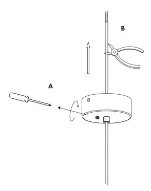
A: REMOVE PLASTIC FROM WIRE. B: WIRE IS NOW READY TO BE CONNECTED TO LED DRIVER.
