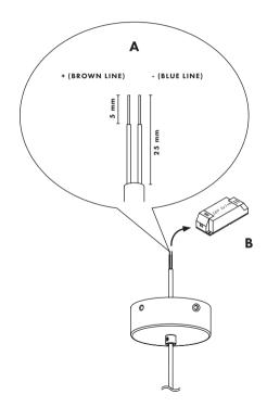
A: TIGHTEN SCREW. B: CONNECT WIRES IN LED DRIVER.
